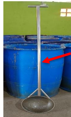
Photo C4: Shaking Spoon . Shaking Spoon is as long as 170 cm. At the end of the soaking period (after 35 days of soaking), pour the Resin Powder Solution into Distillation Pan (Photo D1).
