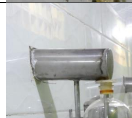
Photo D3: Cooling Hand . Cooling Hand is a tube that placed across Cooling Sink (Photo D4). It connects Distillation Pan (Photo D1) and Oil-Glass Container (Photo D2). Through the Cooling Hand, vapor and oil come Distillation Pan to Oil-Glass Container.
