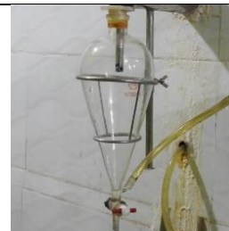
Photo D2: Oil-Glass Container . The Oil-Glass Container is used for stockage oil and water vapor that come from the Distillation Pan (Photo D1). Then, oil and vapor are separated.
