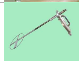
Photo D5: Shaking Stick . Shaking Stick is used for the whole period of distillation. It is connected to cover of the Distillation Pan. About three (03) hours apart, the stick should be shaking during period of distillation.
