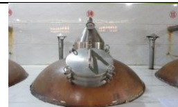
Photo D1: Distillation Pan . Distillation Pan is used for distillation of oil from the Resin Powder Solution. Two containers (Photo C2) of Resin Powder Solution feed into one Distillation Pan and boil it.
