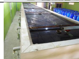
Photo D4: Cooling Sink . Cooling Sink stocks cool water; through which oil (and small amount of vapor) is cooling down before reaching Oil-Glass Container.
